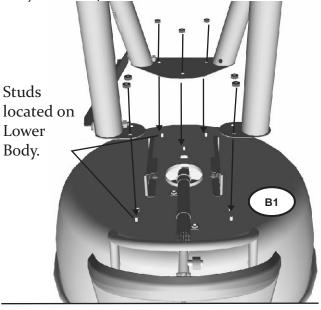
**Step 2** - With the legs assembled to the **Lower Body**, tighten the 4 screws holding the **Cart Bracket** in place. Once complete, turn the grill over to the upright position.
